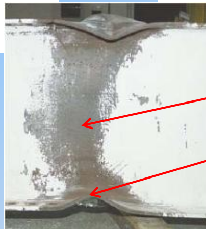
Plastic Collapse Mechanism Experimental Plastic hinge
