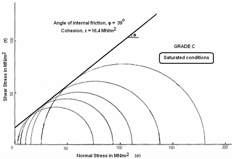
*Figure 11f. Mohr's circles and failure envelope for Grade C - Saturated.*
