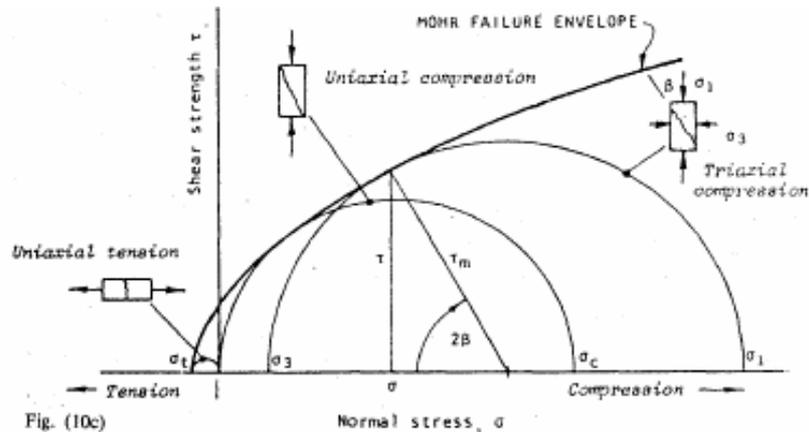
Fig. (10c) Graphical representation of stress conditions for failure of intact rock.
