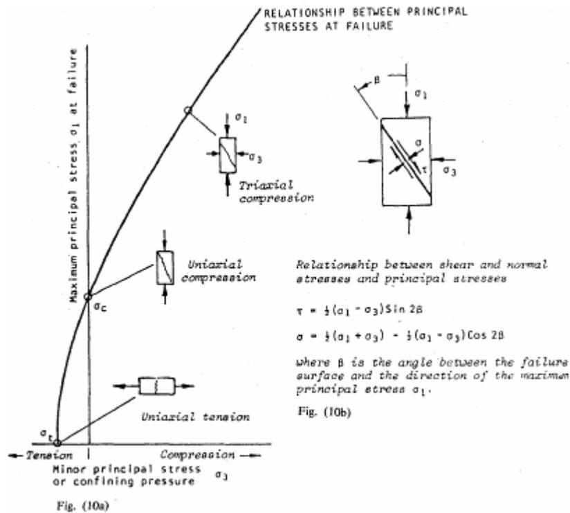
The uniaxial compressive strength of the specimen is given by substituting  $\sigma_3 = 0$  in the equation 1, giving:
