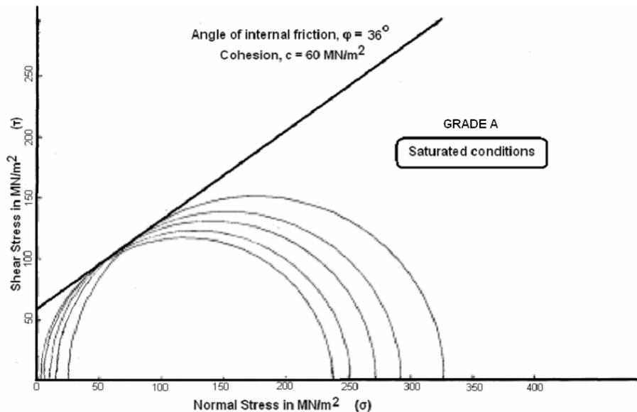
Figure 11b. Mohr's circles and failure envelope for Grade A - Saturated.
