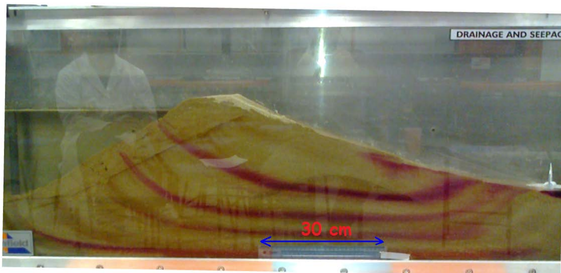
Figure 2: The experiment set up of the earth dam model. Seepage flowlines through the earth dam model are shown.
